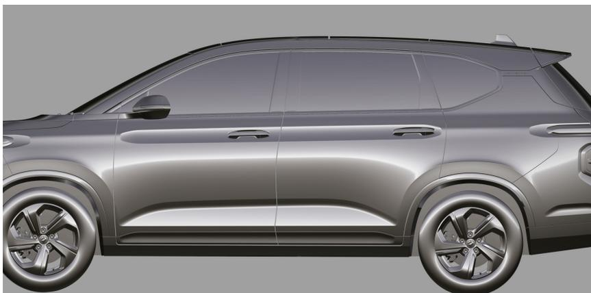
**Fig. 1 Baojun RM-5 door panels in side view (Alias 3D model). The nature of the highlights formation in the area of the shoulder line and doors is clearly demonstrated**
